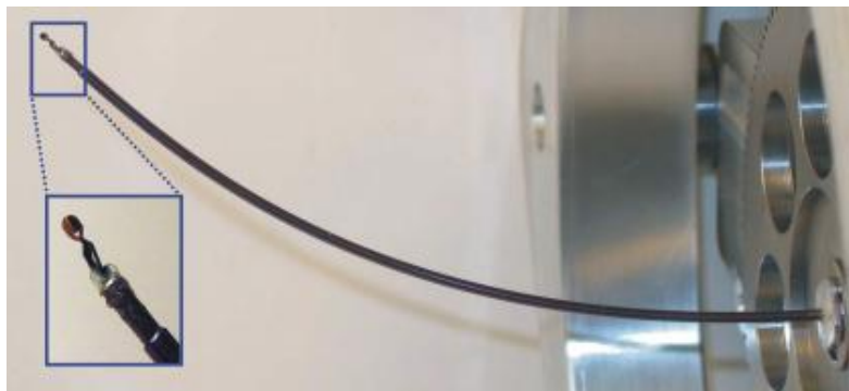
Millimeter-scale forceps protruding from a robotic needle
