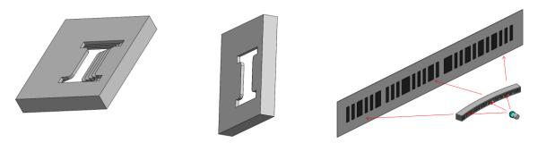
Fig. 6. CAD model of angle-sensitive 3-D device viewed at an arbitrary angle (left); viewed correctly, showing a clean letter "I" (center); concept for projection of a microscale barcode pattern onto a large surface (right).
