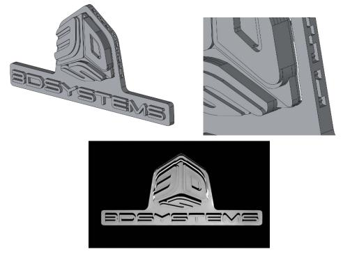
Fig. 5. CAD model of backlit 3D Systems logo structure (top left); close-up view of gap between logo edge and back surface (top right); photograph of the logo with backlighting.
