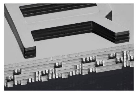
Fig. 3. Barcodes on the vertical sides of the device shown in Fig. 1.
