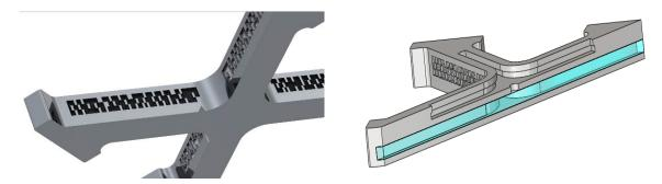
Fig. 7. CAD image of anticounterfeiting device (left); Sectional view of device showing Internal light guide (right)
