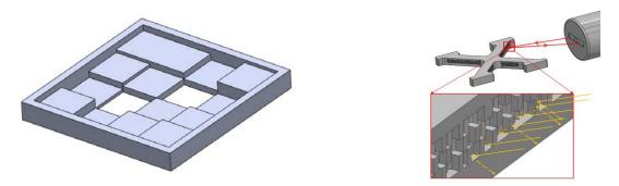
Fig. 4. CAD model of a representative 3-D barcode enabled by MICA Freeform (left); reading a micro 2-D barcode on the side of a device (right).
