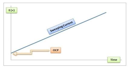
Figure 1. Illustration of a theoretical OCP (Open Circuit Potential).
